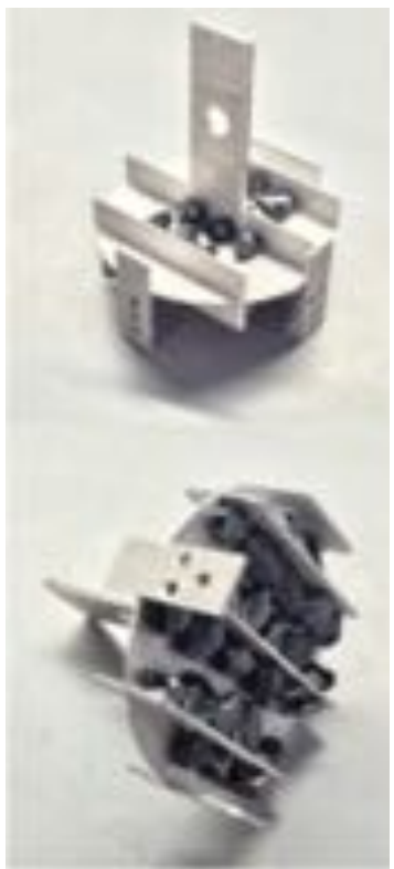
50 co-aligned crystals m = 5.1 g mosaic < 2^\circ
